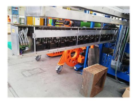
Digital inkjet solution to prevent vulcanisation of rubber textiles for production of inflatable boats
