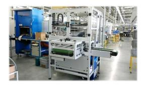
Production line assembled from 10 components with 2 ultrasonic welding stations for VW / Audi
